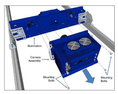
Figure 127: Removing the camera
