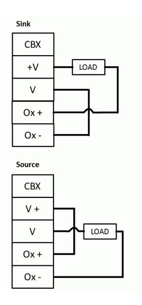
**Figure 76: Powered Output Connections**
