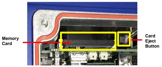
Figure 124: Memory card and eject button location
