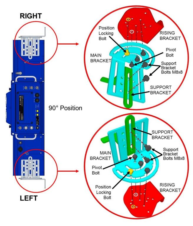
Figure 29: Side Bracket Assembly, Top=Right Mounting (90°)
