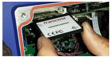
Figure 125: Removing the memory card
