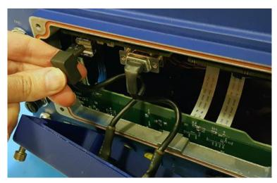
Figure 92: Connecting USB Cable
