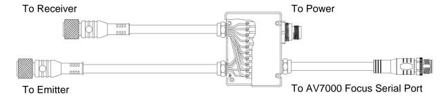
Figure 115: CVL-2403 Connection Cable
