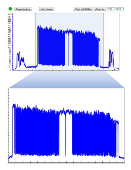
9. Click **Next Step >>>.** The **Step 2/5 Mounting Calibration Window** opens. The AV7000 uses the image and determine the optimal far working distance for the camera. This step takes a while and the "Please Wait" message will blink during this time.
