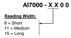
Figure 9: AI7000 Illumination Model Description Key
