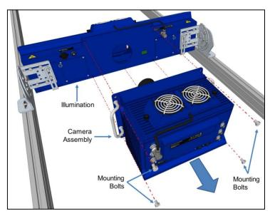
Figure 122: Removing the camera
