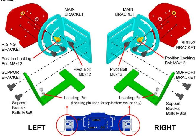
Figure 26: Bracket Assembly for Top and Bottom Mounted Cameras (Exploded View 90°)
