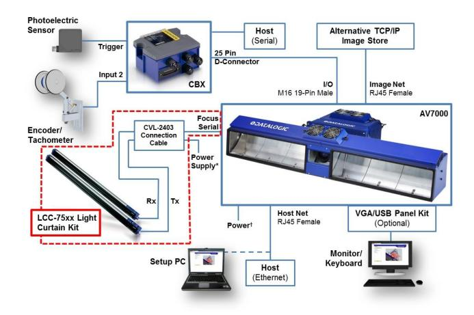
Figure 53: Single AV7000 with LCC-75xx Light Curtain Kit
