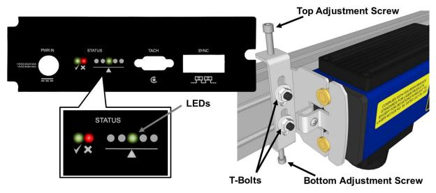
Figure 107: RangeFinder Leveling
