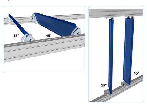
Figure 48: Alternative Deflection Mirror Mounting Between Rails
