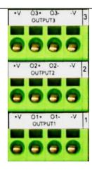
Figure 84: OUTPUTS Block
