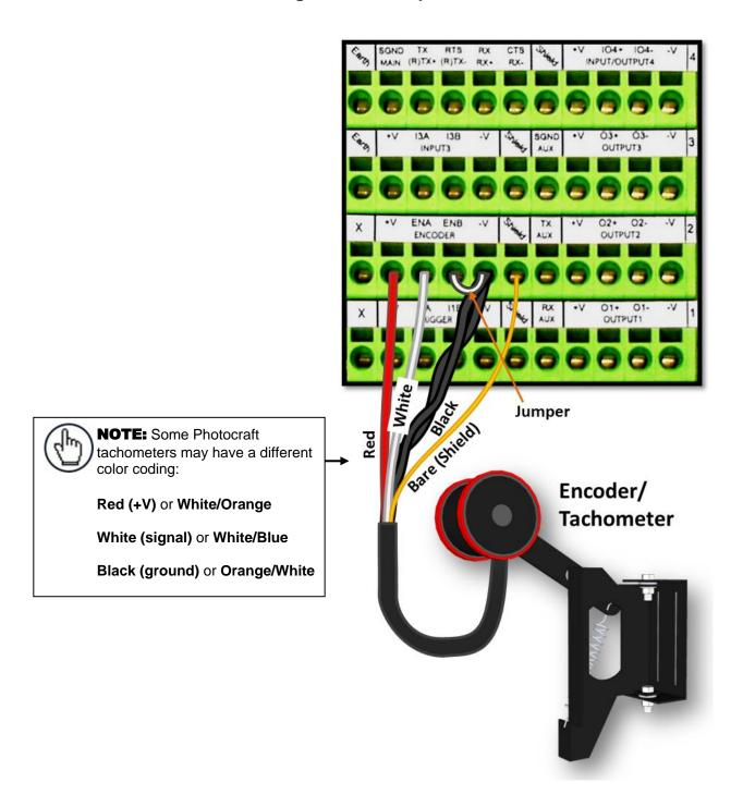
Figure 82: OEK-2 (93ACC1770) Encoder/Tachometer Wiring (PNP Output)
