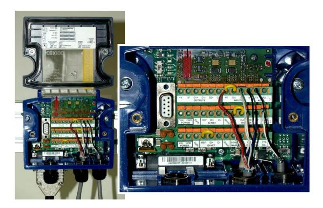
Figure 62: Securing wires with water-tight seals
