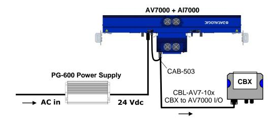
Figure 60 - Connecting PG-600 to Al7000 Illuminator
