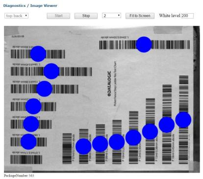
5. Continue running the box and making adjustments until the barcodes are in focus. Make sure that barcodes from both columns have been read.
