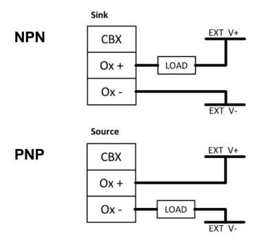
Figure 85: Unpowered Outputs
