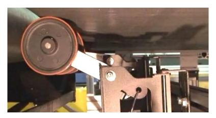
Figure 147: Tachometer Wheel
