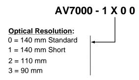
Figure 8: AV7000 Camera Model Description Key
