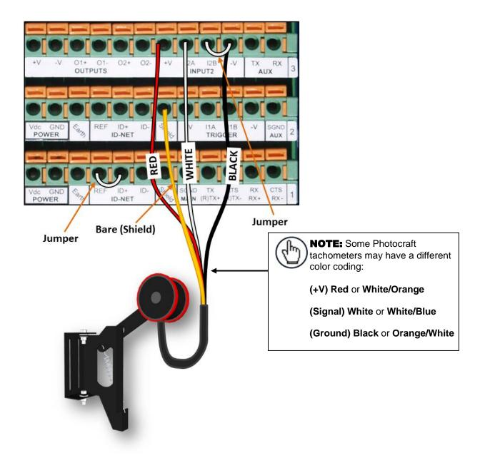
Figure 70: OEK-2 Encoder/Tachometer Wiring (PNP Output)
