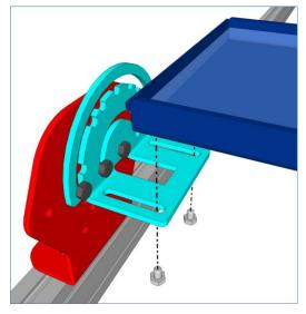
Figure 41: Top mirror mounting position
