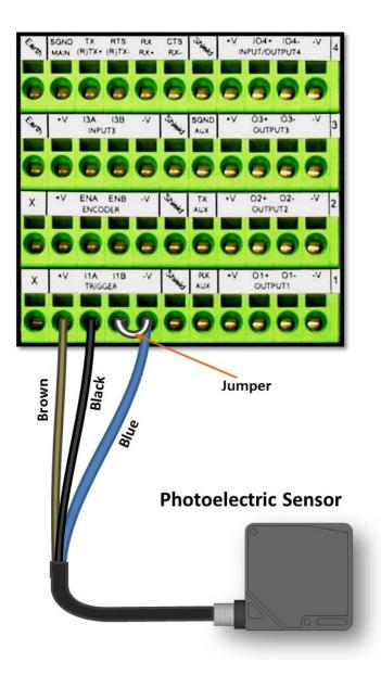
Figure 79: Photoelectric Sensor Wiring (PNP Output)
