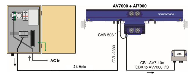
Figure 61 - Connecting PWR-480B to Al7000 Illuminator
