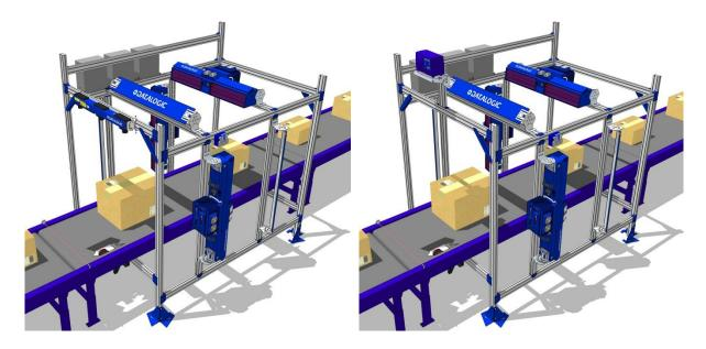
Figure 5: Typical Reading Station with RangeFinder (left) and DM3610 (right)
