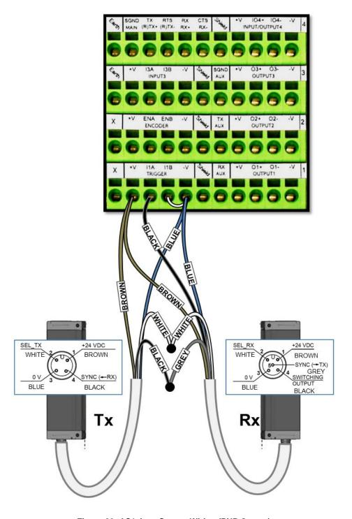
Figure 80: AS1 Area Sensor Wiring (PNP Output)
