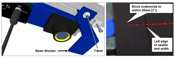
Figure 108: Installing Beam Blockers (LEFT) and Close-up of the RangeFinder's scan line pattern along edge of conveyor (RIGHT)
