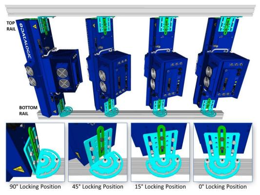
Figure 35: Alternative Mounting: SIDE Camera Between Rails
