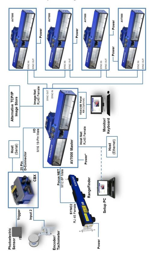
Figure 55: Master/Slave Array (Tunnel) with RangeFinder
