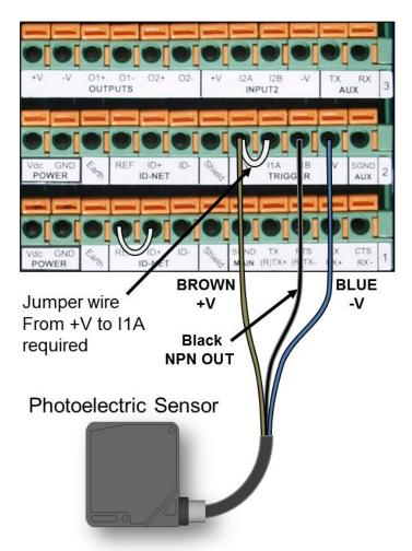
Figure 66: Photoelectric Sensor Wiring (NPN Output)
