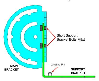
Figure 25: Mounting Support Bracket with short bolts
