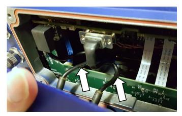
Figure 93: Carefully positioning the USB and VGA cables
