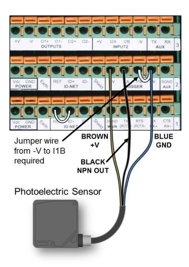
Figure 67: Photoelectric Sensor Wiring (PNP Output)
