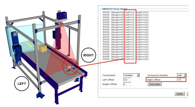
Figure 103: Right Side Box/Spacer Width Calculation
