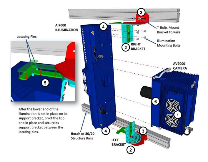
Figure 31: Mounting a SIDE AV7000 Camera
