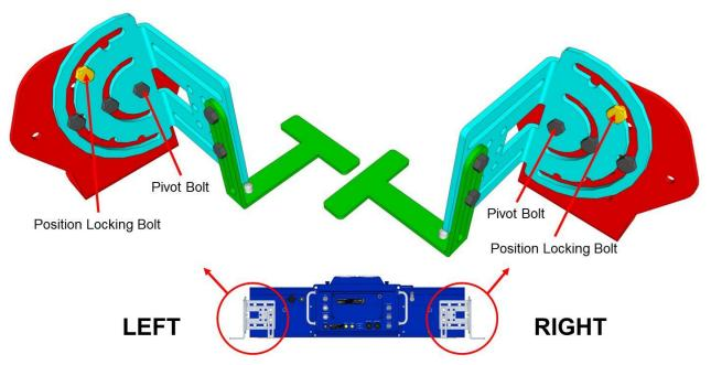
Figure 27: Bracket Assembly for Top and Bottom Mounted Cameras (Assembled 90°)
