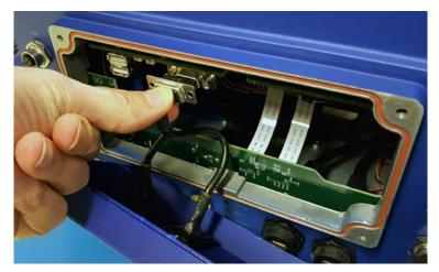
Figure 91: Connecting VGA Cable
