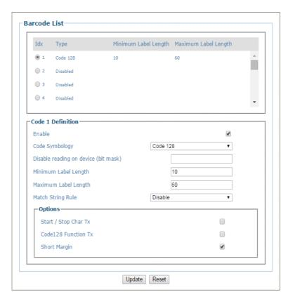
2. Set the barcode menu to read the **Picket Fence/Step Ladder Res Test Chart** (code 128 barcodes).
