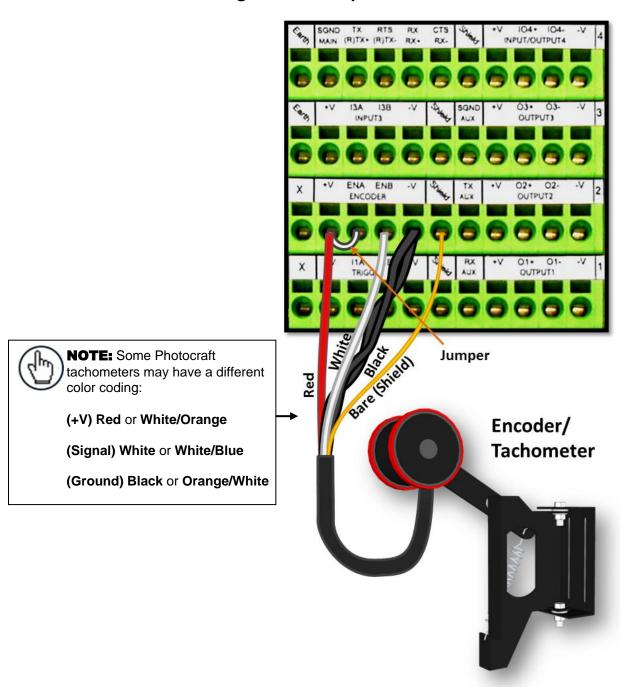
Figure 81: OEK-2 Encoder/Tachometer Wiring (NPN Output)
