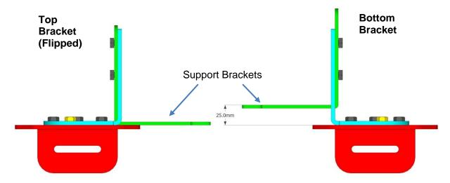
Figure 30: Side Bracket Assembly, Support Bracket position
