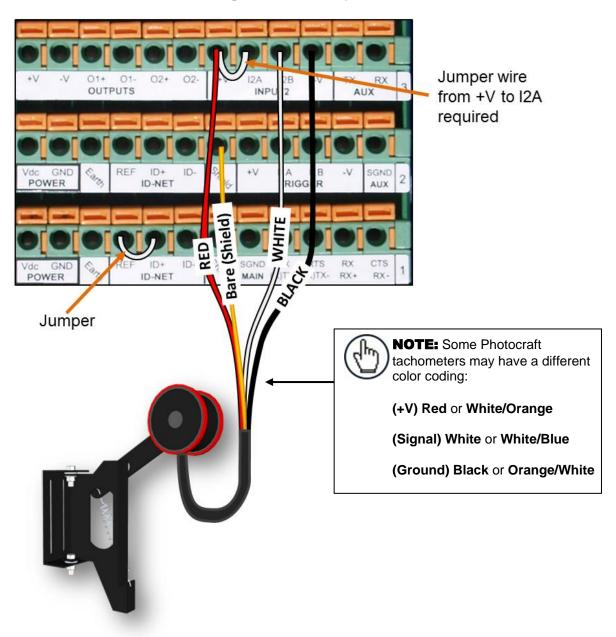
Figure 69: OEK-2 Encoder/Tachometer Wiring (NPN Output)
