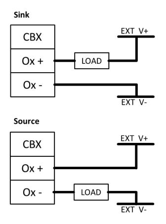
**Figure 75: Unpowered Output Connections**
