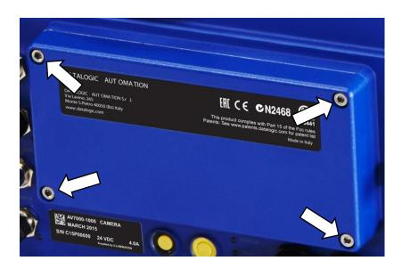
Figure 89: Rear access panel screw locations
