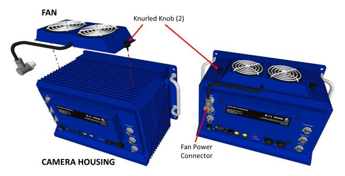
Figure 36: Mounting the cooling fan to the AV7000 Camera
