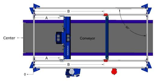
Figure 49: AV7000 with Deflection Mirror Mounting/Alignment (TOP VIEW)
