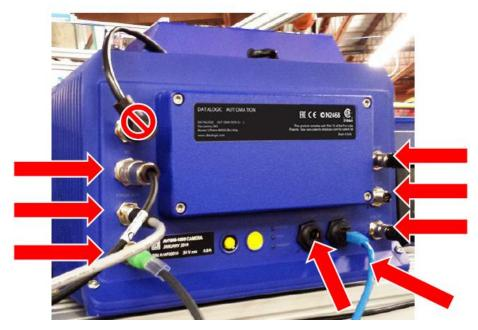
Figure 126: Remove the cables
