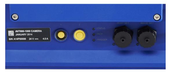
Figure 10: AV7000 External Function Buttons
