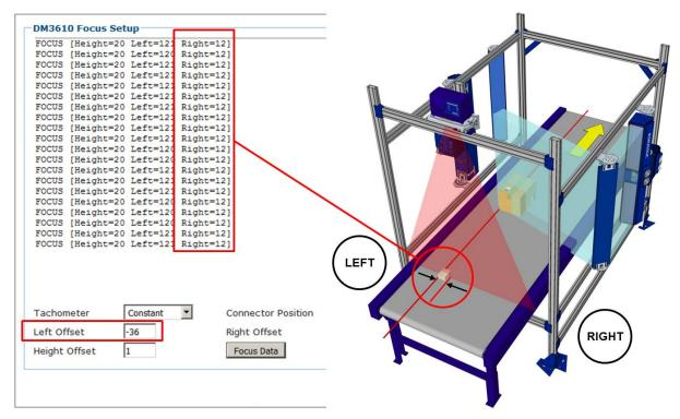
Figure 101: Left Side Box/Spacer Width Calculation
