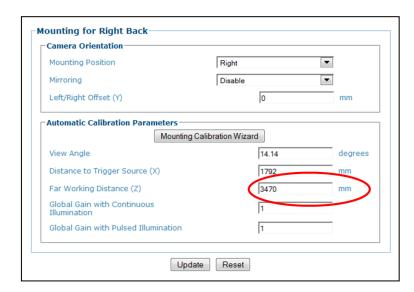
4. Adjust the **Far Working Distance (Z)** parameter incrementally and run the box through the system again.
