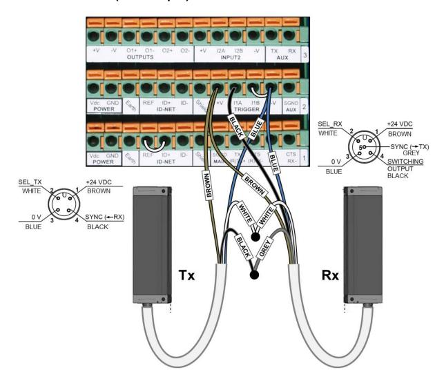
Figure 68: AS1 Area Sensor Connections (PNP Output)
