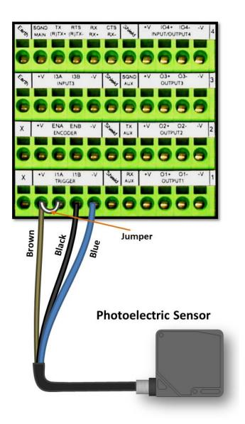
Figure 78: Photoelectric Sensor Wiring (NPN Output)
