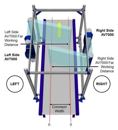
Figure 96: Conveyor Width
