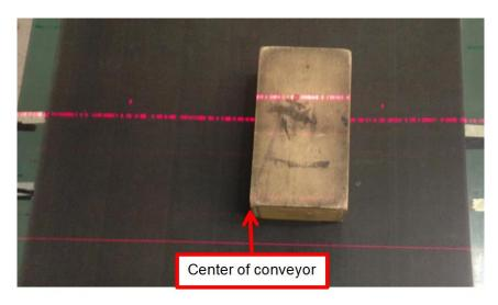
Figure 112: Box of known height placed in RangeFinder scan line
