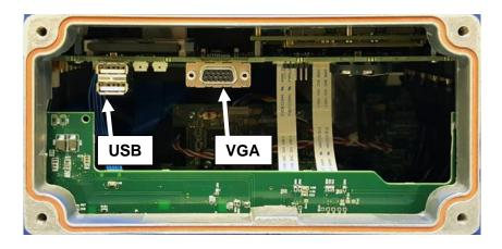
Figure 90: USB and VGA Connectors inside camera
