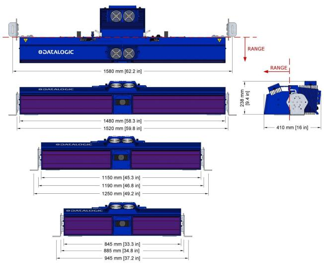
**Figure 21: Mounting Dimensions**
