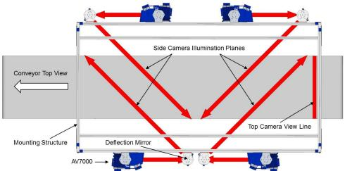
Figure 6: Multi-Camera Station with Standard Continuous Illumination
