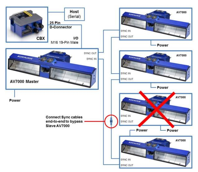
Figure 149: Bypassing a slave AV7000
