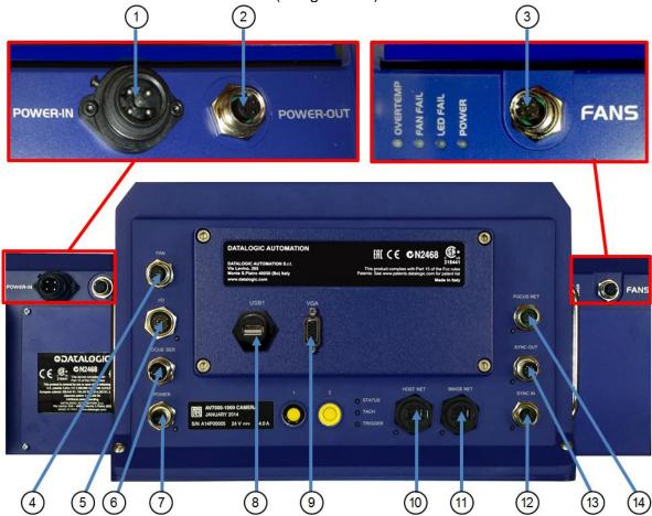
Figure 57: AV7000/AI7000 Connector Panels
