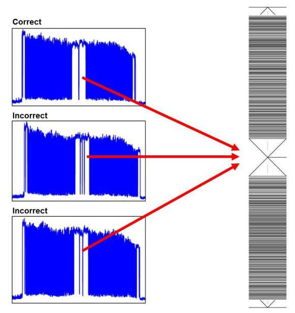
Figure 117: Focus Target Position
