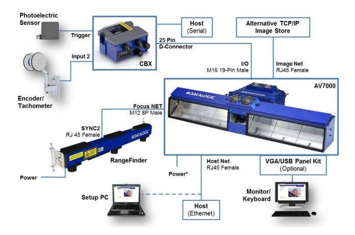
Figure 52: Single AV7000 with RangeFinder
