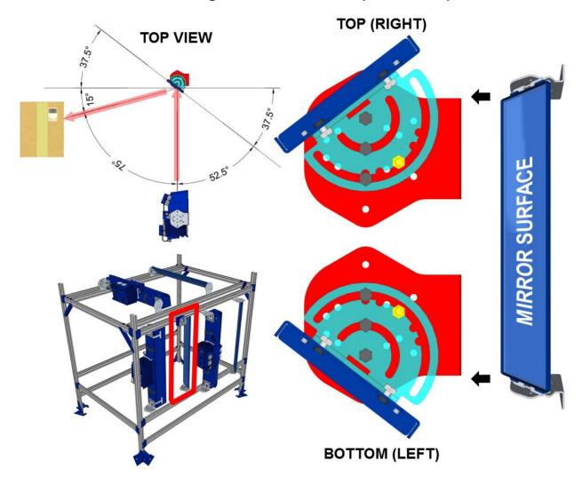
Figure 46: 15° View Angle with Old Bracket Inside Side
