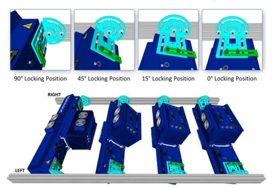
Figure 34: Alternative Mounting: TOP Camera Between Rails
