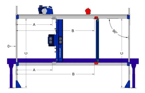
Figure 50: AV7000 with Deflection Mirror Mounting/Alignment (SIDE VIEW)
