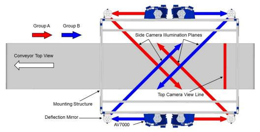
Figure 7: Multi-Camera Station with Pulsed Illumination
